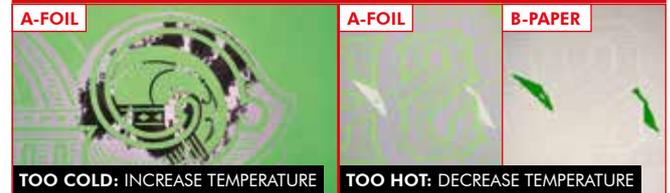
**IMPORTANT:** Different printer manufacturers use different types of toner. The settings above are only reference values! Finding out the optimal temperature and time requires trial and error.
